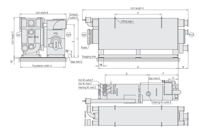
HTG Enlarged  $H_3$ ,  $H_4$  dimensions (HTG Enlarged  $H_1$ ,  $H_2$  is the same size with standard models) (Refer to P24 of the DFA standard model for dimensions not shown in the drawing)
