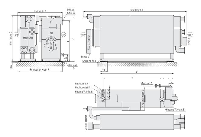
HTG Enlarged  $H_3$ ,  $H_4$  dimensions (HTG Enlarged  $H_1$ ,  $H_2$  is the same size with standard models) (Refer to P23 of the DFA standard model for dimensions not shown in the drawing)
