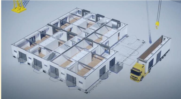
The Installation and Transportation Process of 5D Building
